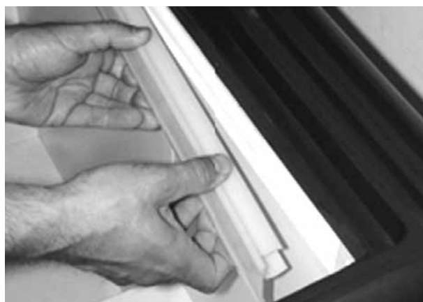
Fig. 6: Remove lamp cover
