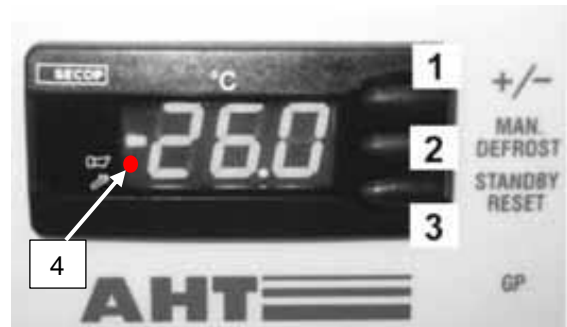
Fig. 3: Electronic controller, operating elements and screen displays
