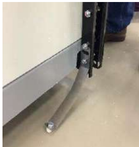
Fig. 7.2: Device-specific tilt protection
