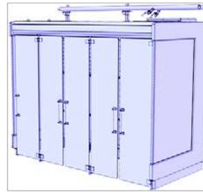
Fig. 11: “ROLL-IN” device with glass doors (GD) in closed state
