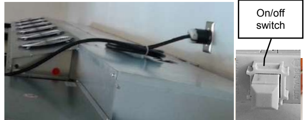
Fig. 8.2: Device connection 208-240V network and ON/OFF switch (symbol display)
