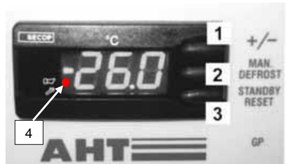
Fig. 3: Electronic controller, operating elements and screen displays
